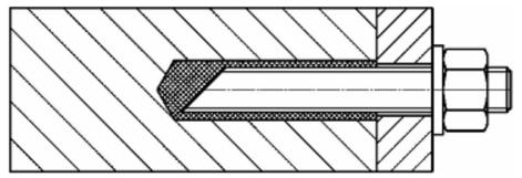
Standard threaded rod with two side 45° chamfer
