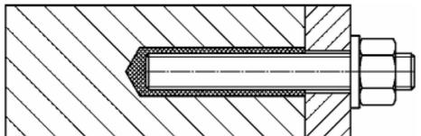
Standard threaded rod with one side 45° chamfer
